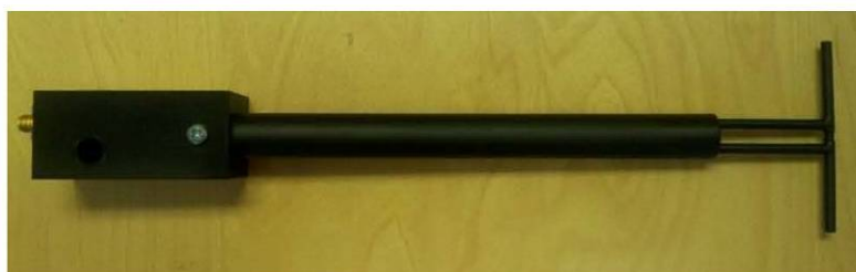
Figure 1 – MVG COMOSAR Validation Dipole
