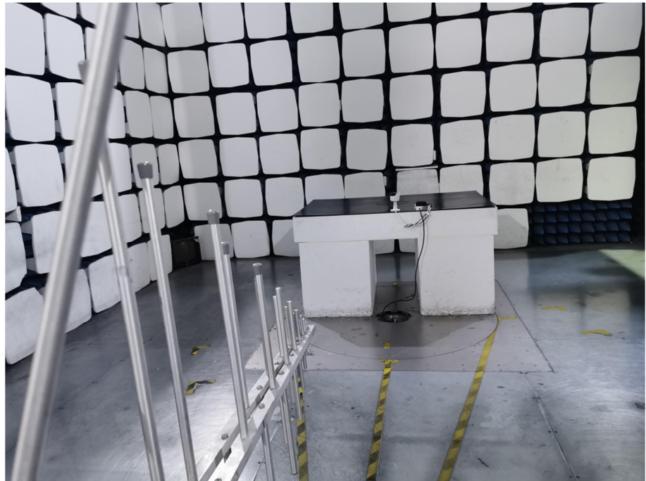
Radiation Emission Test Setup (30MHz to 1GHz)
