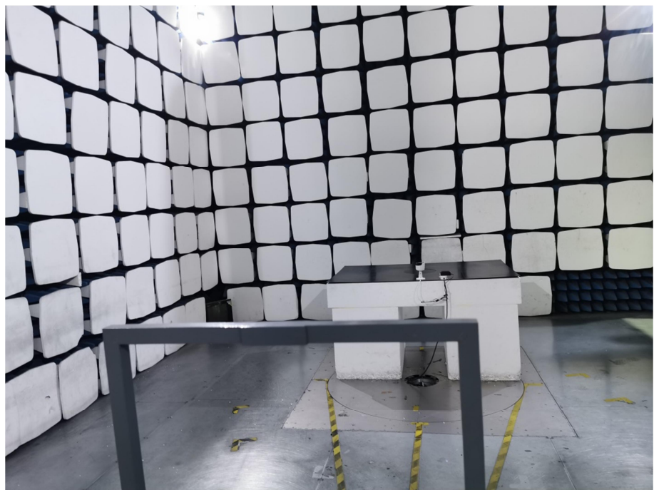
Radiation Emission Test Setup (Below 30MHz)
