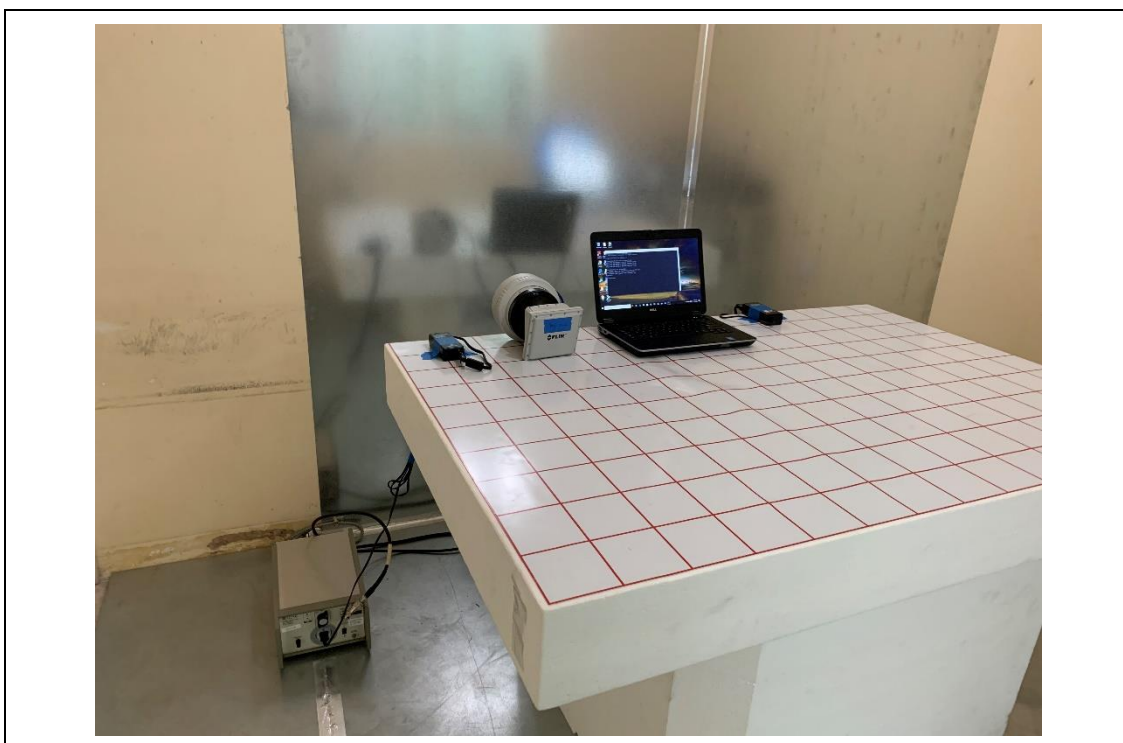
AC Line Conducted Emission setup – Front
