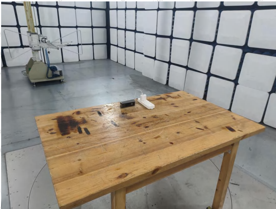
Photo of Radiation Emission Test
