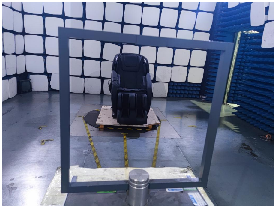
Radiation Emission Test Setup (Below 30MHz)
