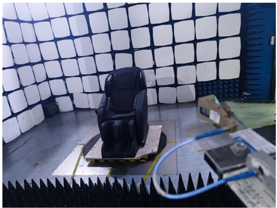
Radiation Emission Test Setup (Above 18GHz)
