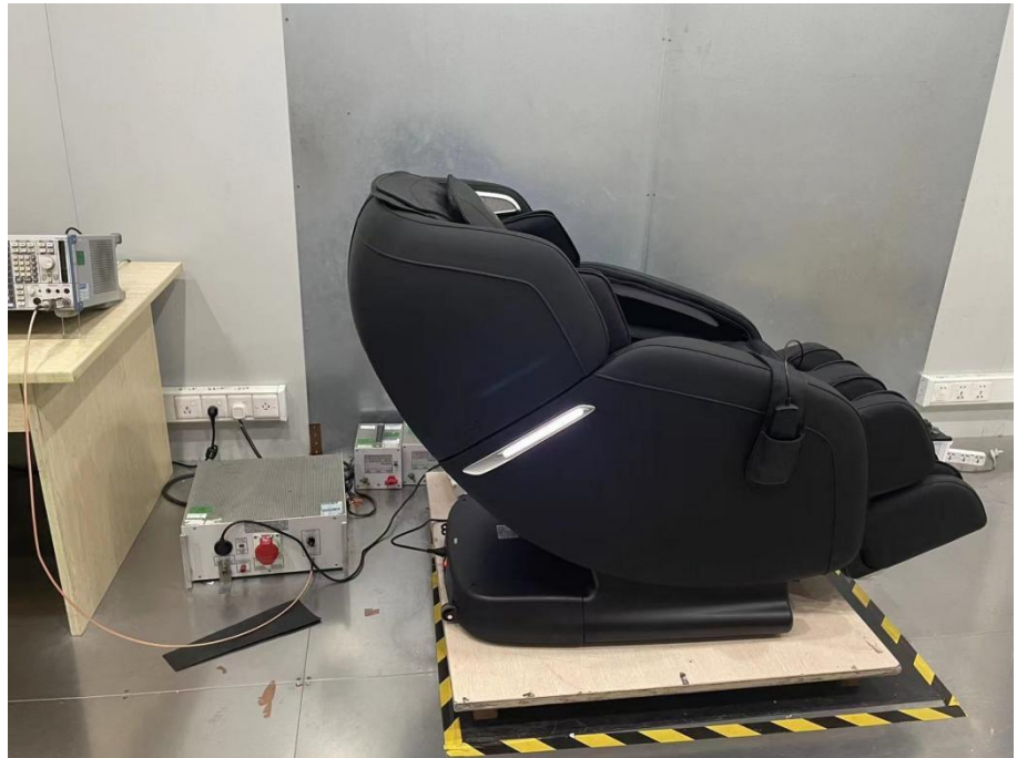
Conducted Emission Test Setup
