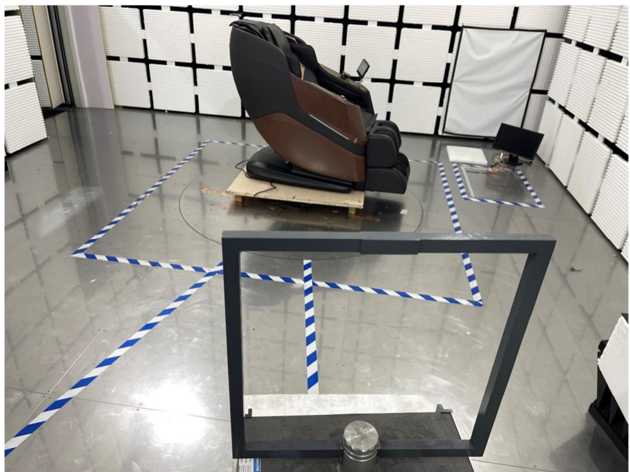
Radiation Emission Test Setup (Below 30MHz)
