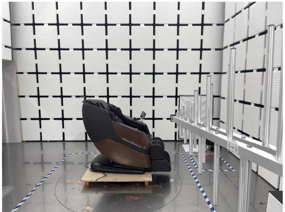
Radiation Emission Test Setup (30MHz to 1GHz)
