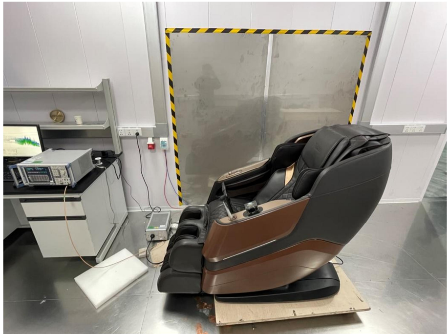
Conducted Emission Test Setup
