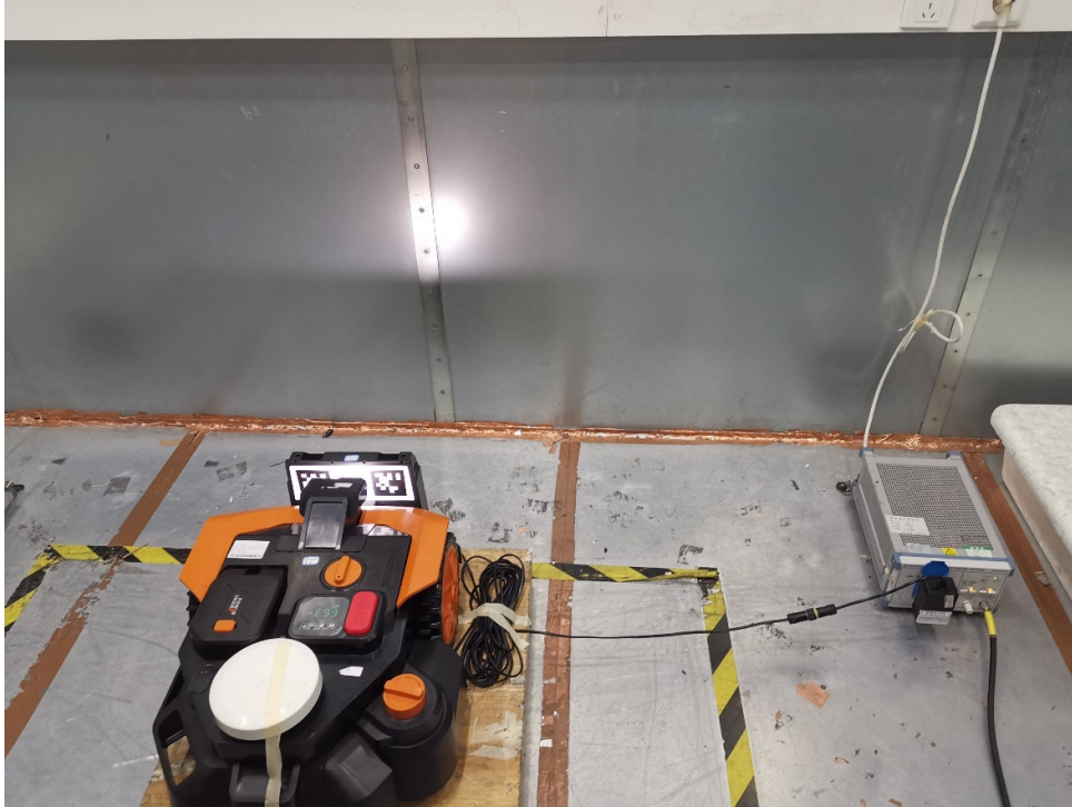
Picture 2 Conducted Emission Test Setup
