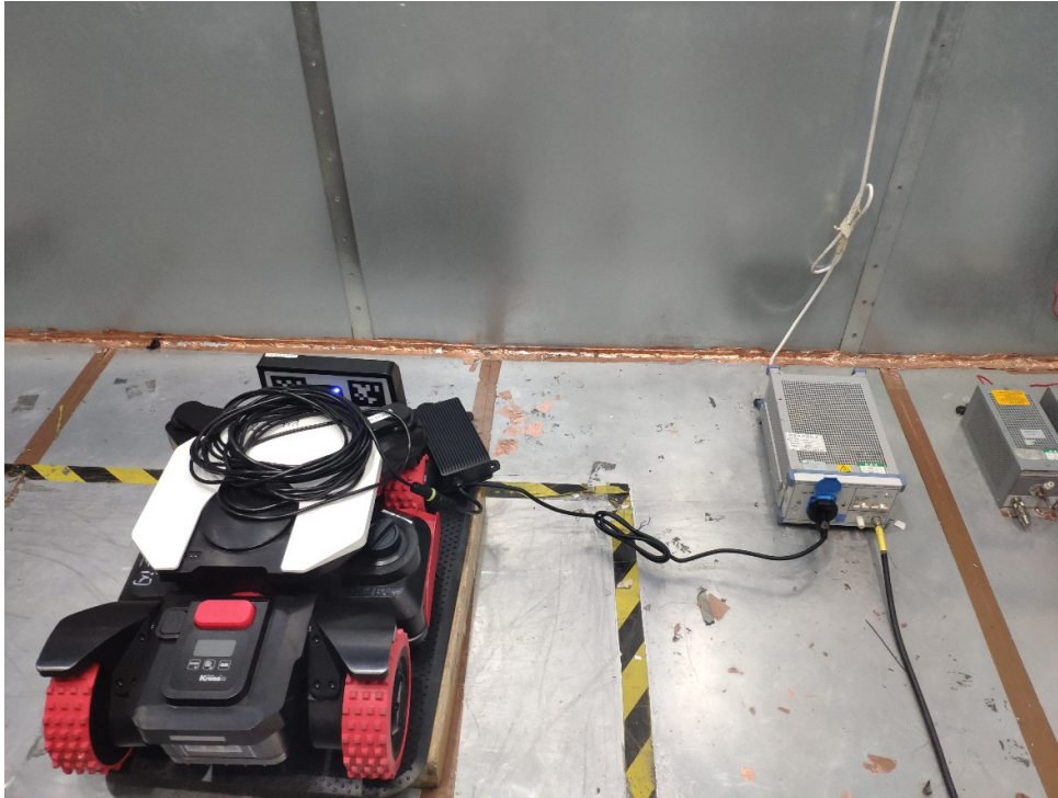
Picture 2: Conducted Emissions Test Setup
