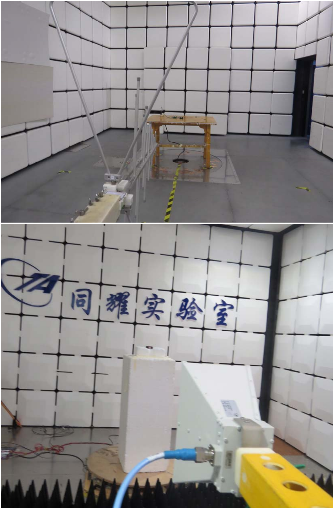
Picture 2 Radiated Spurious Emissions Test setup
