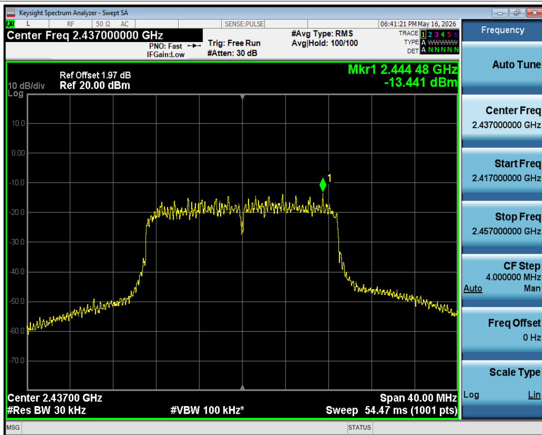
PSD NVNT n20 2437MHz Ant1
