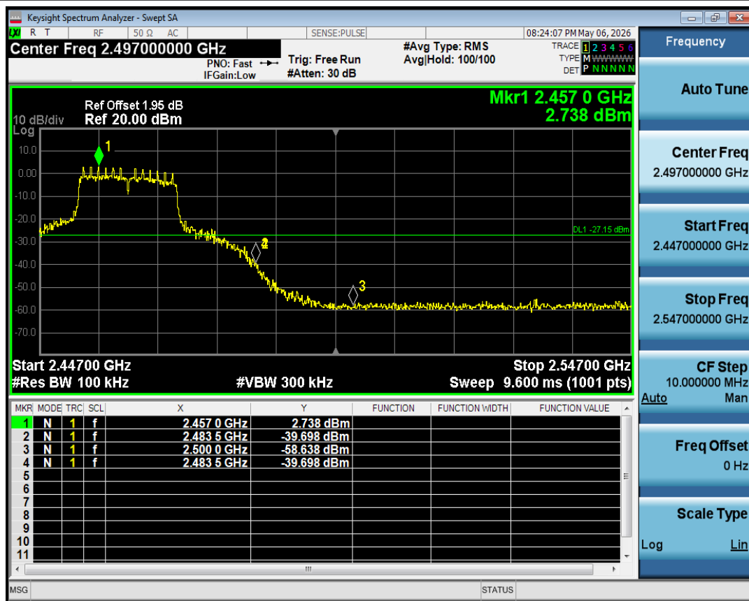
Band Edge NVNT g 2462MHz Ant1 Emission
