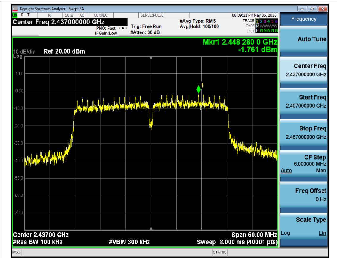
Tx. Spurious NVNT n40 2437MHz Ant1 Ref
