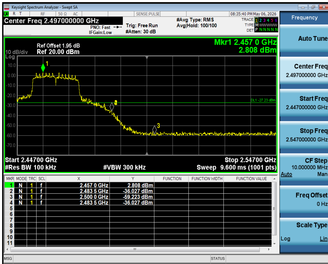
Band Edge NVNT ax20 2462MHz Ant1 Emission
