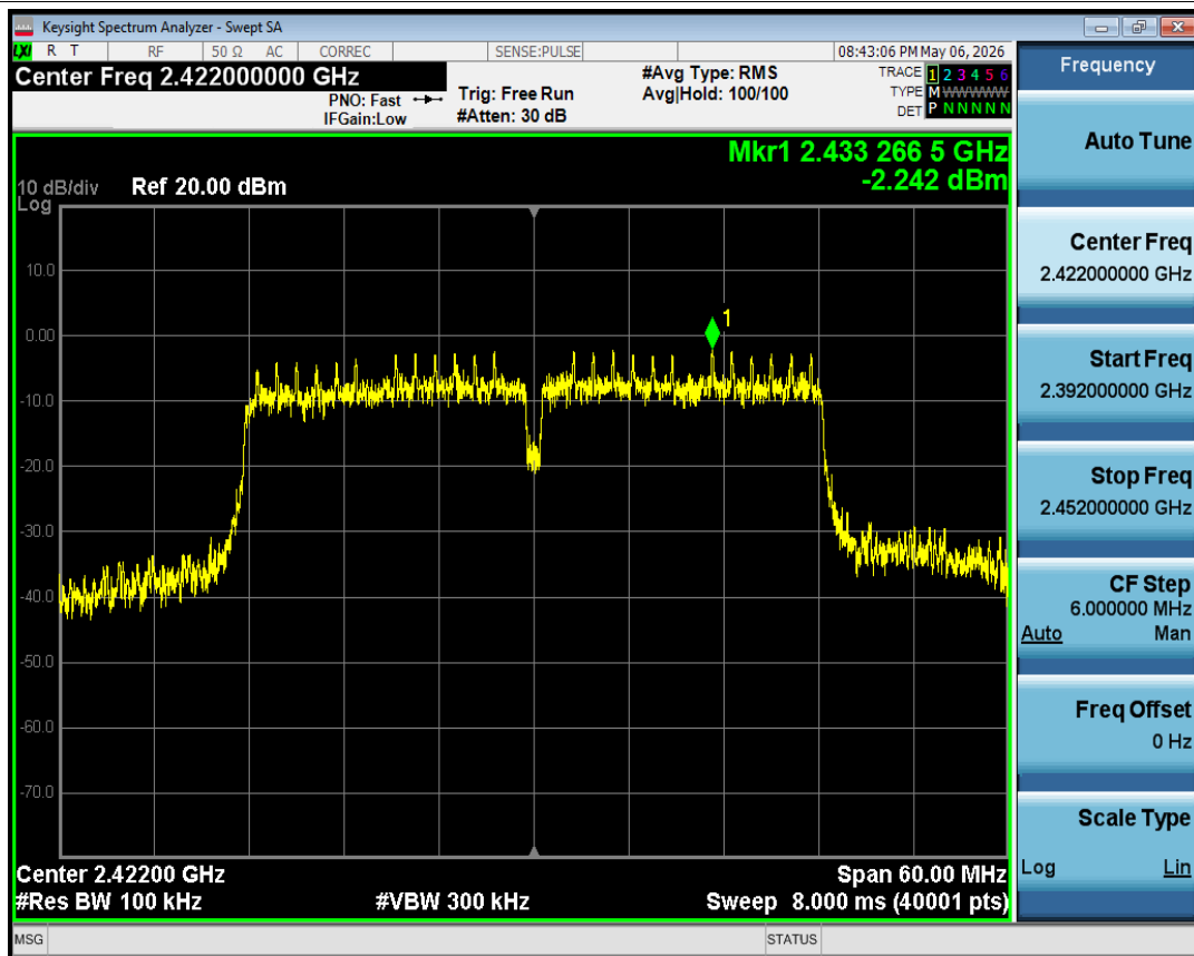
Tx. Spurious NVNT ax40 2422MHz Ant1 Ref
