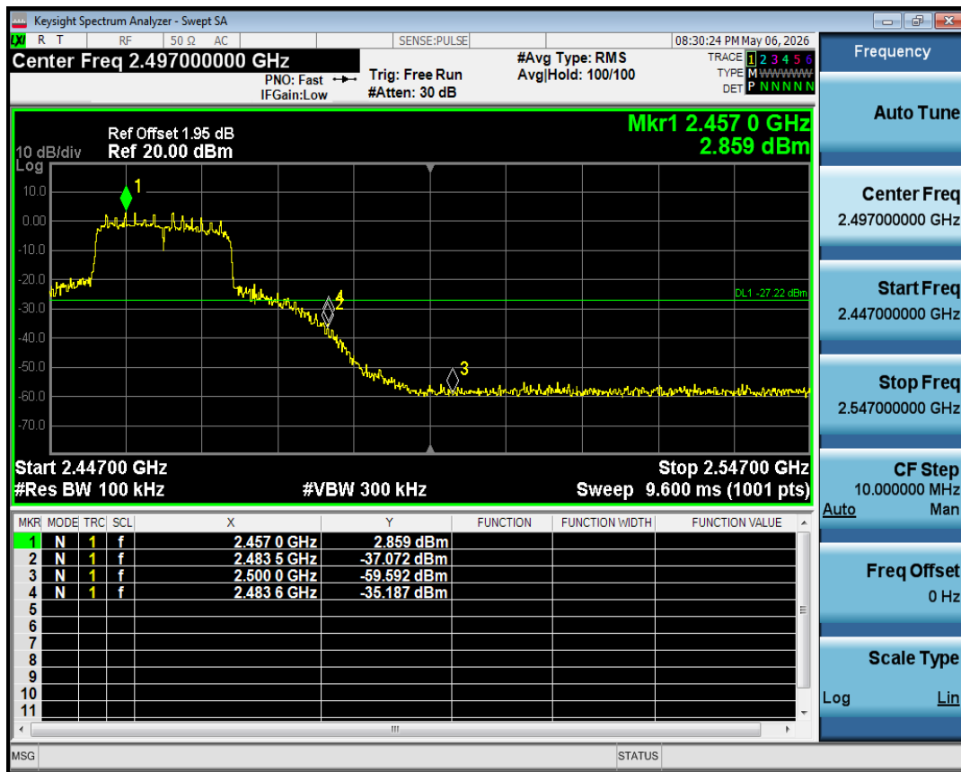
Band Edge NVNT n20 2462MHz Ant1 Emission
