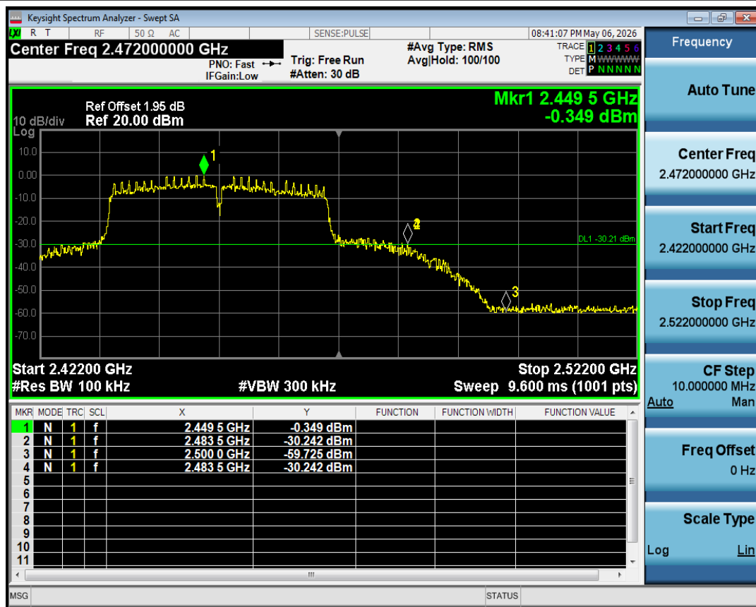
Band Edge NVNT n40 2452MHz Ant1 Emission
