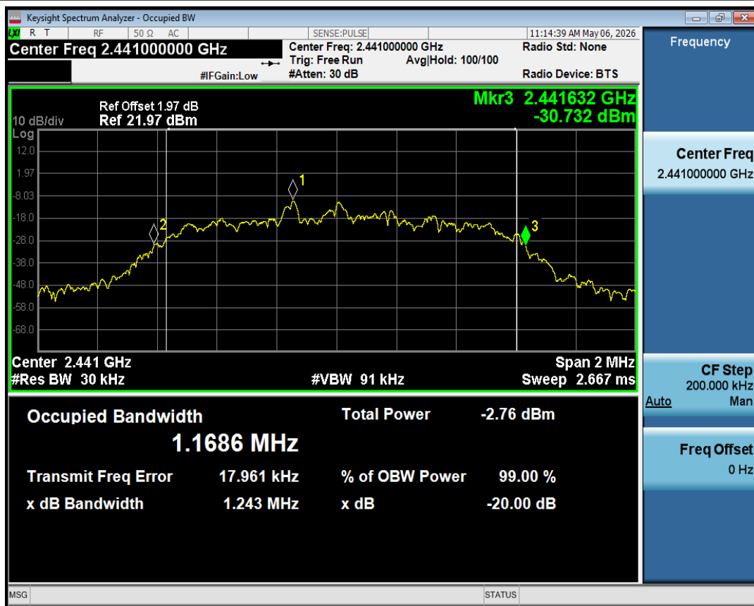
-20dB Bandwidth NVNT 3-DH1 2441MHz Ant1
