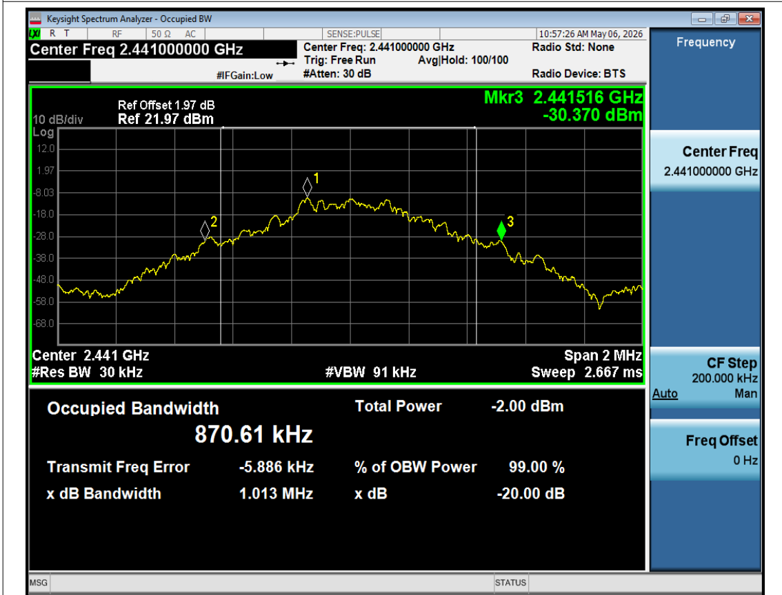
-20dB Bandwidth NVNT 1-DH1 2441MHz Ant1
