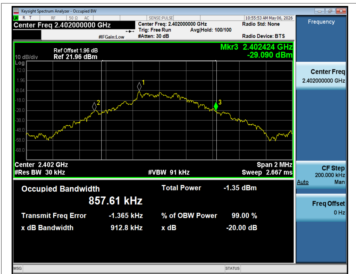
-20dB Bandwidth NVNT 1-DH1 2402MHz Ant1
