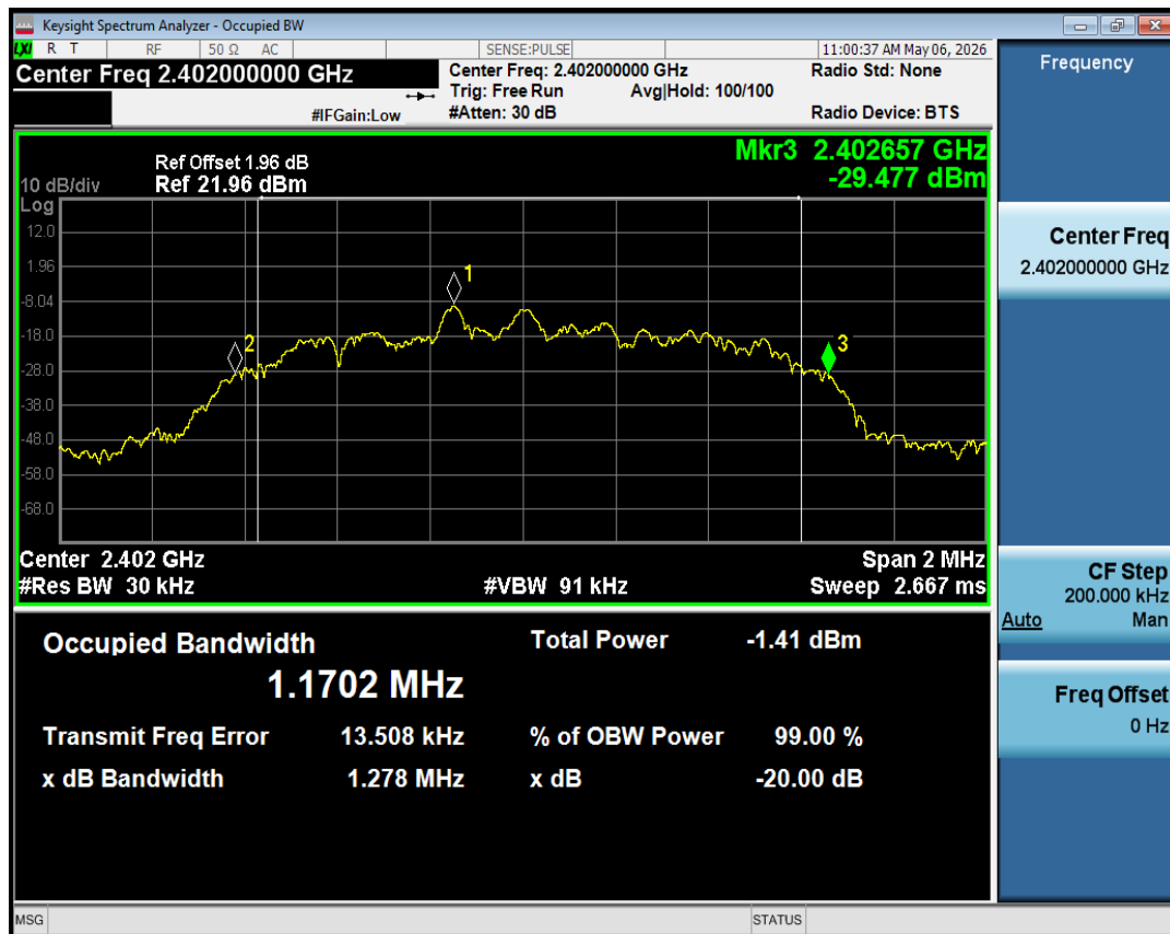
-20dB Bandwidth NVNT 2-DH1 2402MHz Ant1
