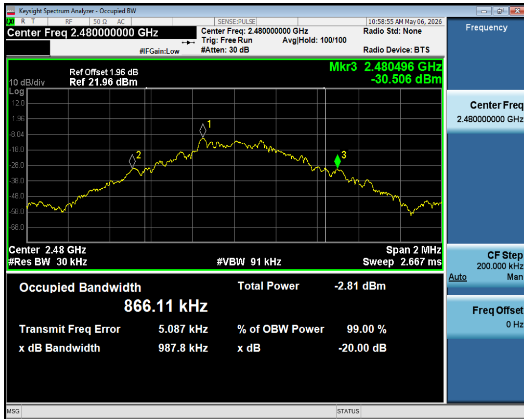
-20dB Bandwidth NVNT 1-DH1 2480MHz Ant1
