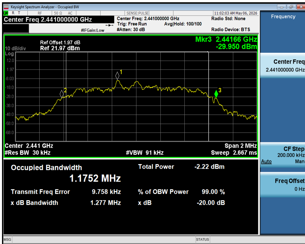
-20dB Bandwidth NVNT 2-DH1 2441MHz Ant1
