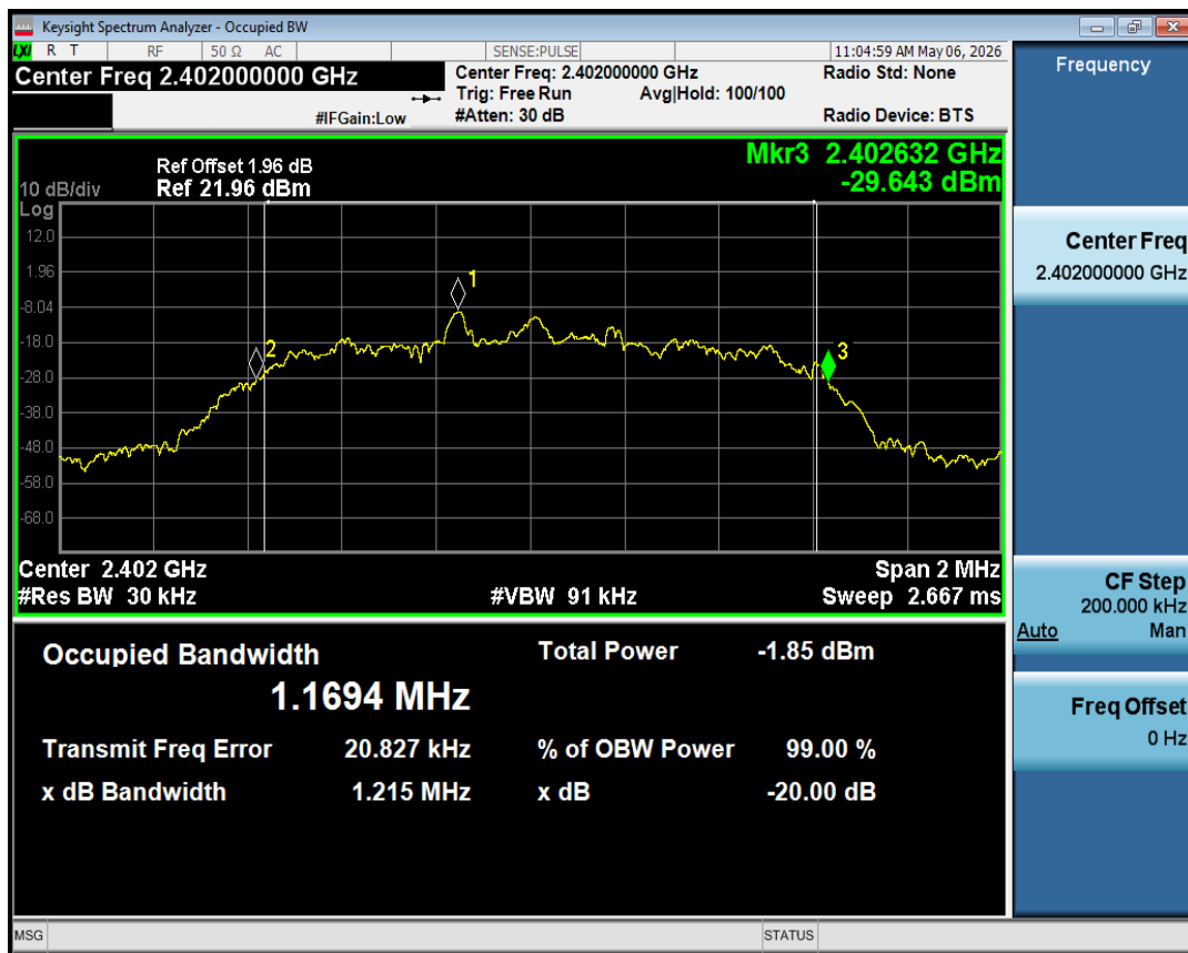
-20dB Bandwidth NVNT 3-DH1 2402MHz Ant1
