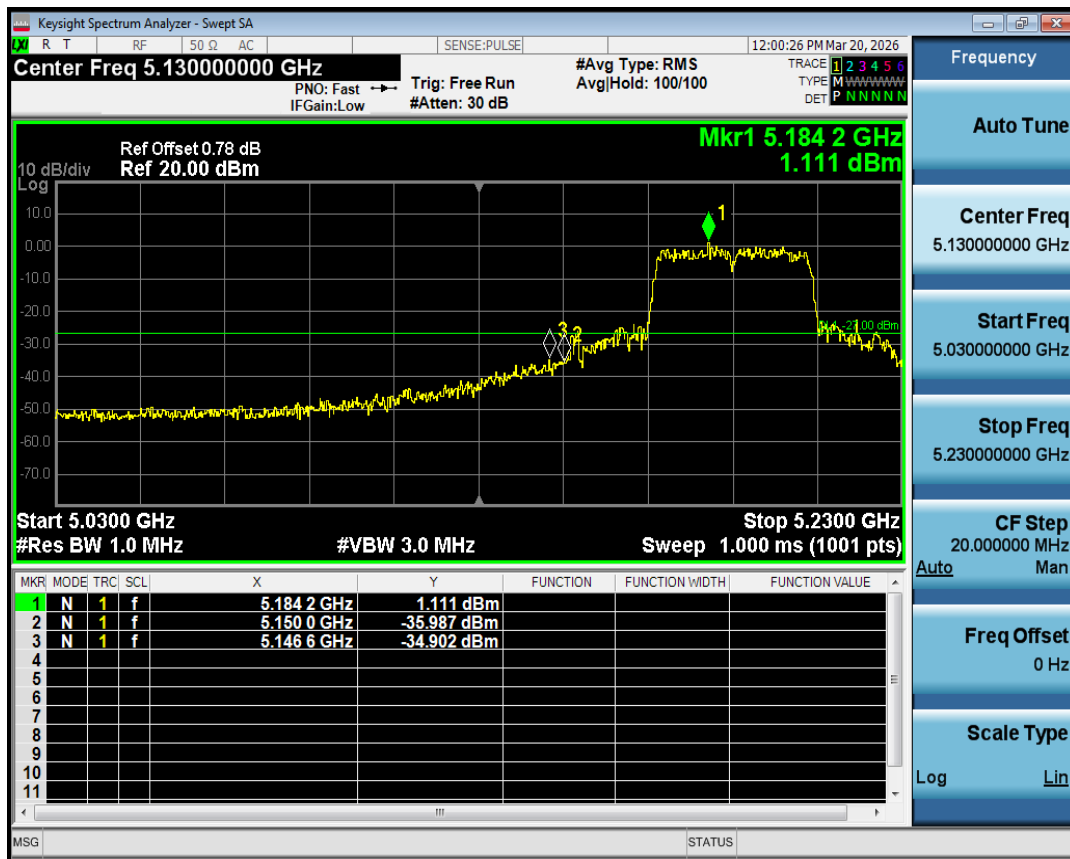
Band Edge NVNT n40 5190MHz Low Ant1
