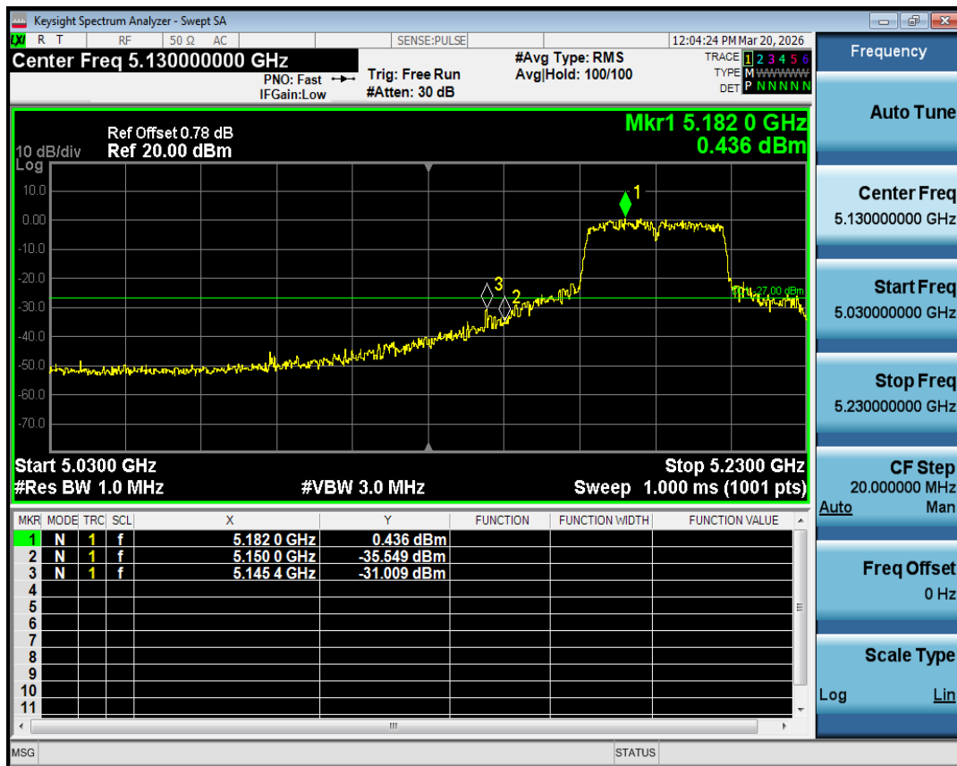
Band Edge NVNT ac40 5190MHz Low Ant1
