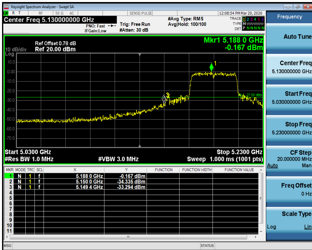
Band Edge NVNT ax40 5190MHz Low Ant1
