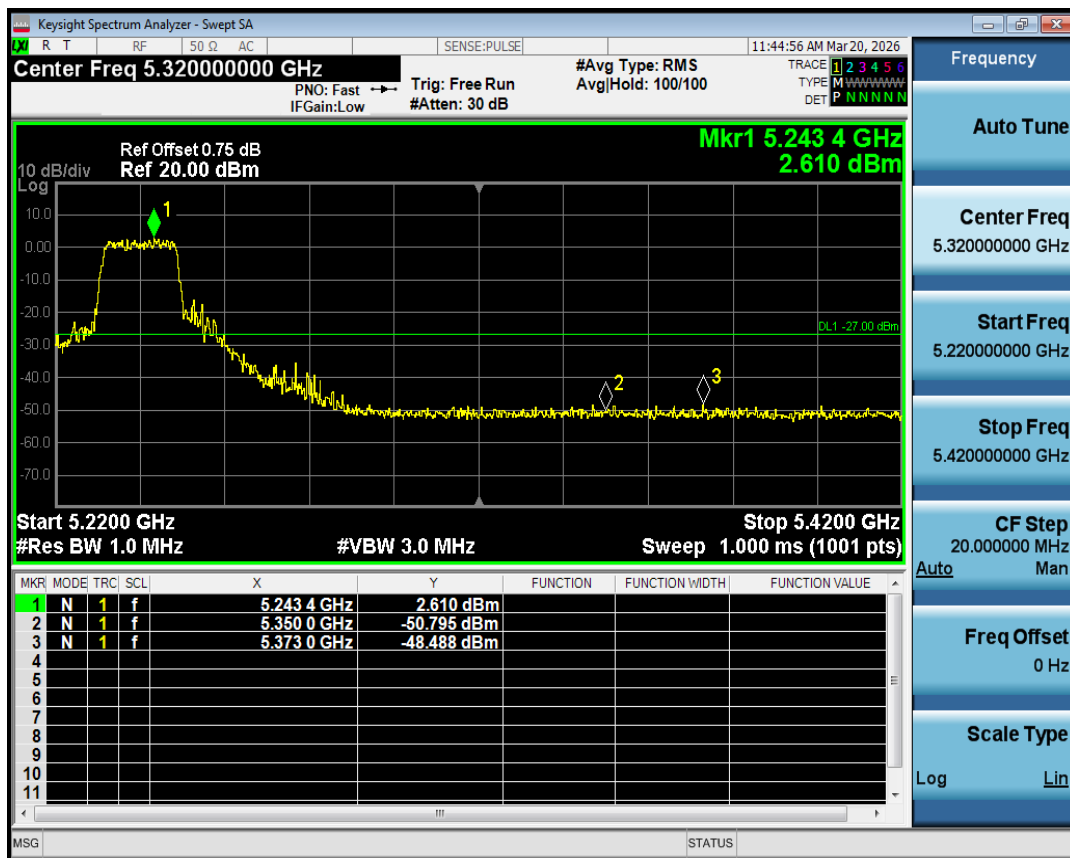
Band Edge NVNT n20 5240MHz High Ant1
