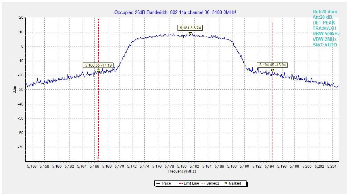
Fig. 10 Occupied 26dB Bandwidth (802.11a, 5180MHz)
