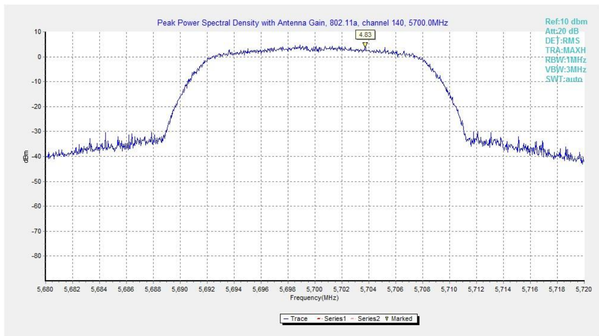
Fig. 9 Power Spectral Density (802.11a, 5700MHz)
