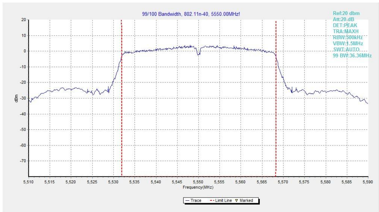
Fig. 50 99% Occupied Bandwidth (802.11n-HT40, 5550MHz)
