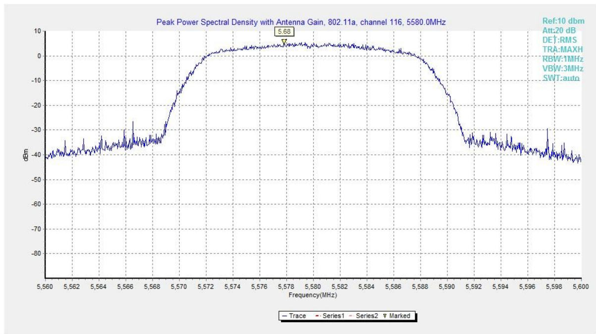
Fig. 8 Power Spectral Density (802.11a, 5580MHz)
