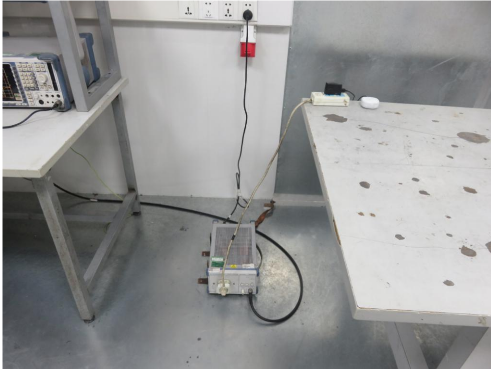
Photo of Conducted Emission Measurement
