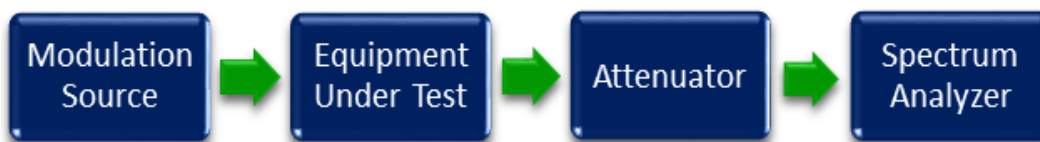
Figure 3: Occupied Bandwidth Test Setup
