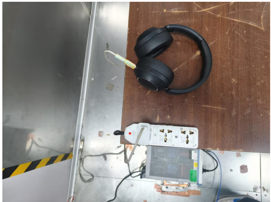
Conducted Emission Test Setup(close up)
