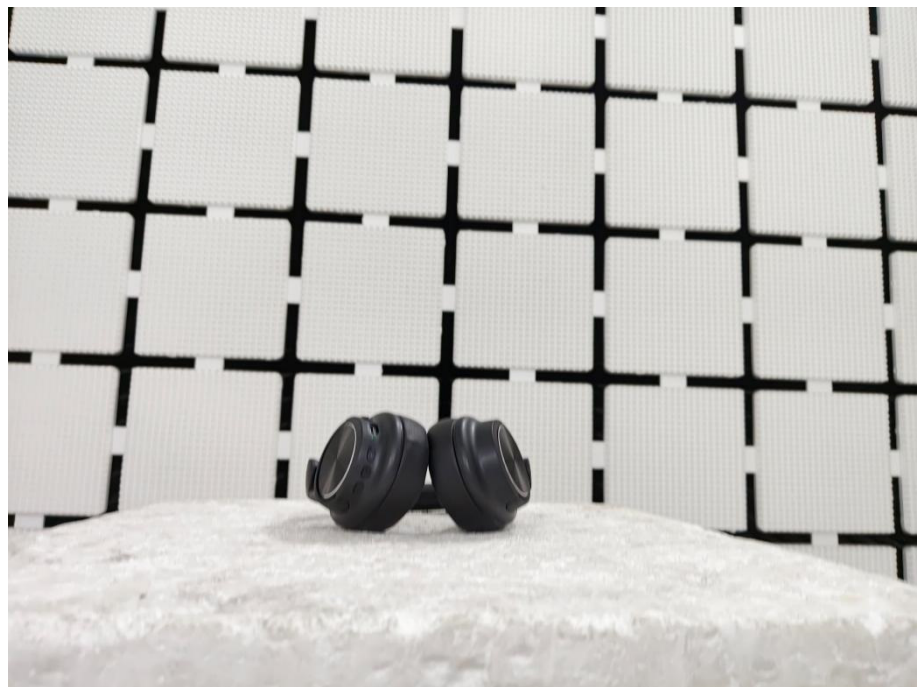
Radiation Emission Test Setup (close-up)
