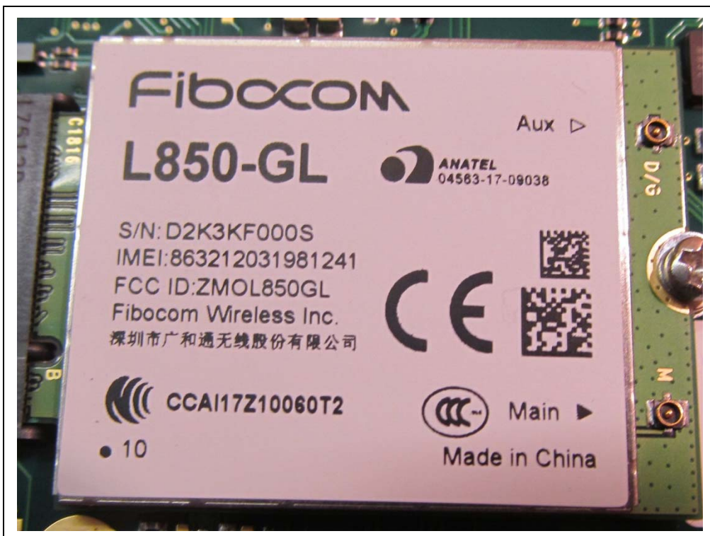
Photograph A3-14: Label of Cellular radio module (on D3 Carrier Board)
