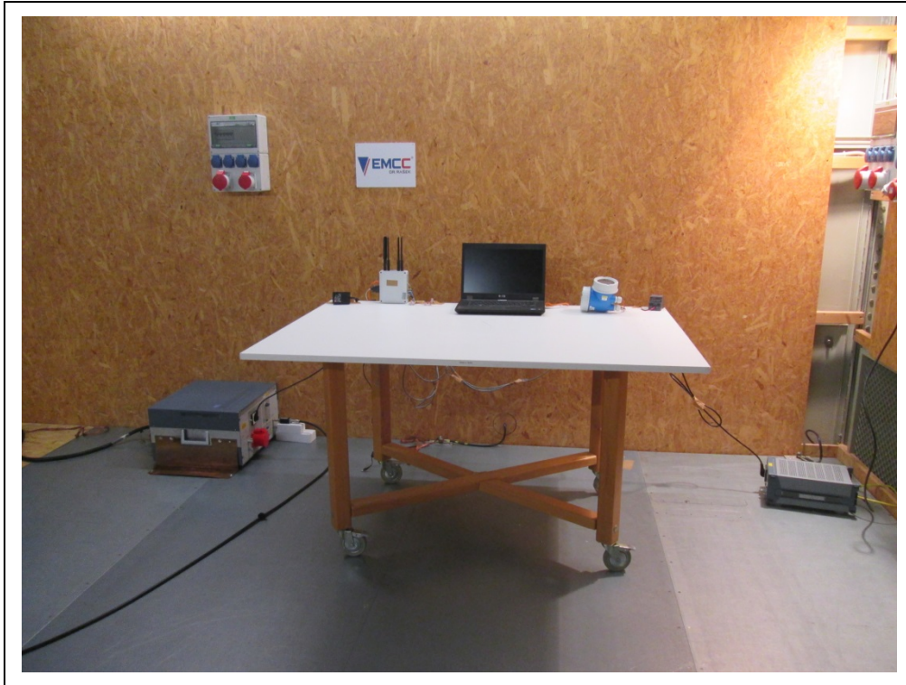
Photograph A1-1: Conducted emissions
