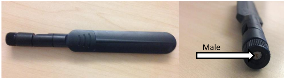
Figure 18: Antennas for LTE and Sub-1GHz networks with SMA Male connector
