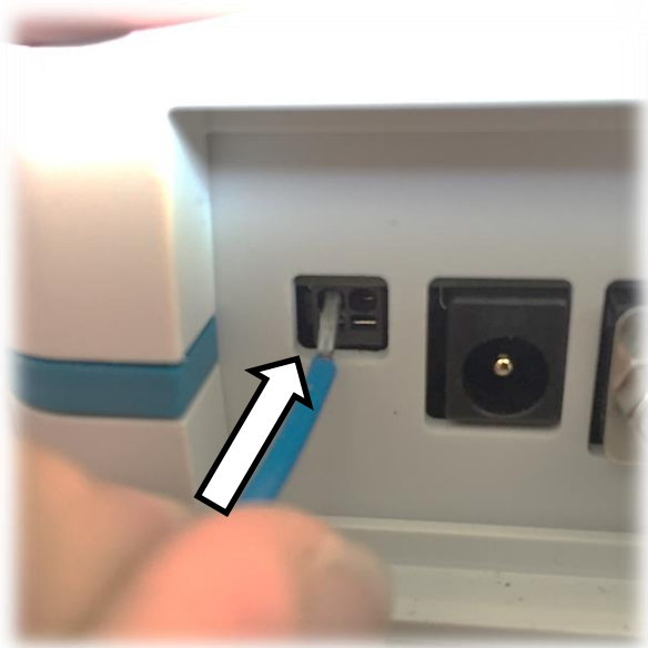
Figure 23: Inserting cable into push-in spring socket
