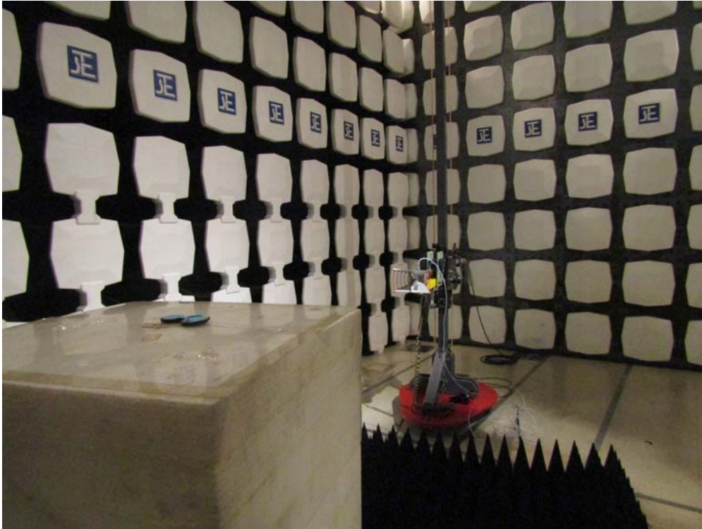
Measurement of Radiated Emission Test Set Up
