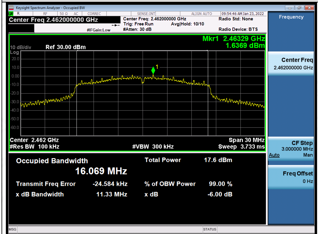
Test_Graph_802.11g_ANT1_2462_6Mbps_DTSBW
