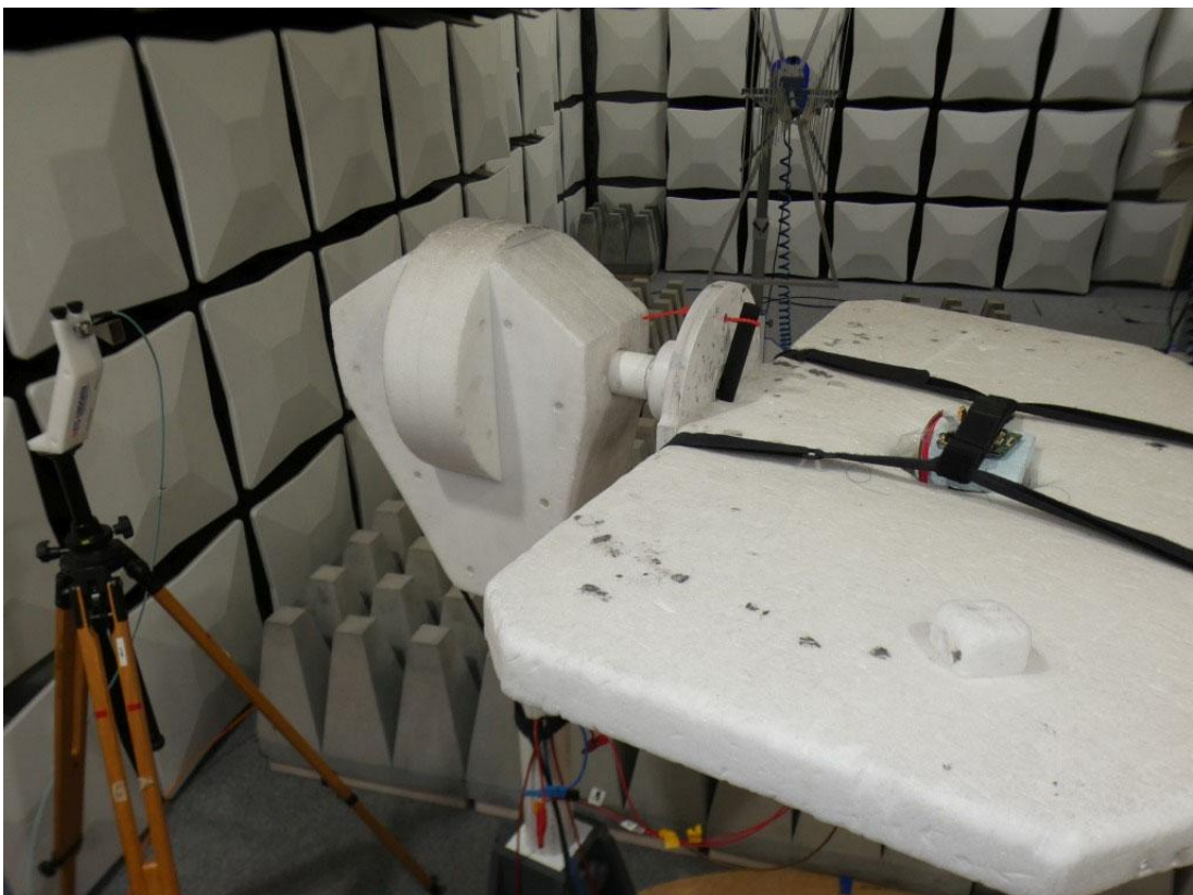
Photo 4: Test setup for radiated measurements above 26 GHz
