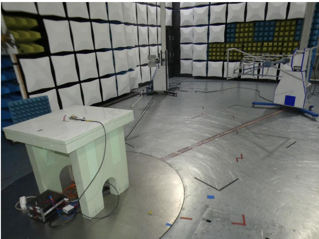
Photo 2: Test setup for radiated measurements below 1 GHz
