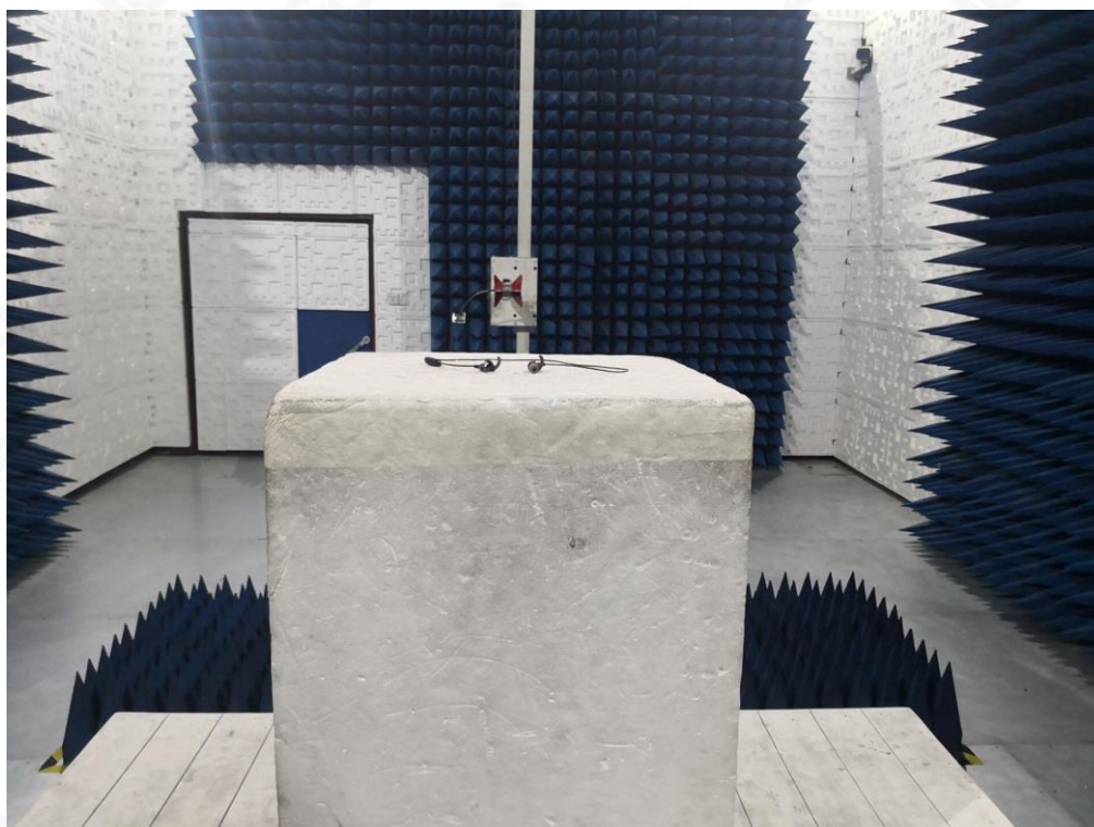
RADIATED EMISSION TEST SETUP ABOVE 1GHZ
