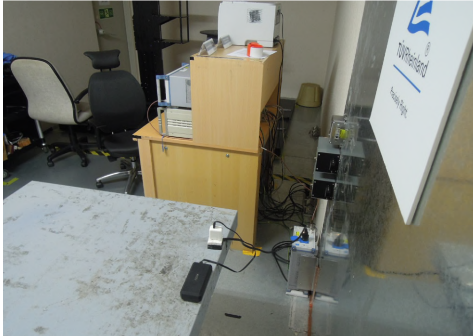
Photograph 16: Set-up for Mains Conducted testing (Back View)
