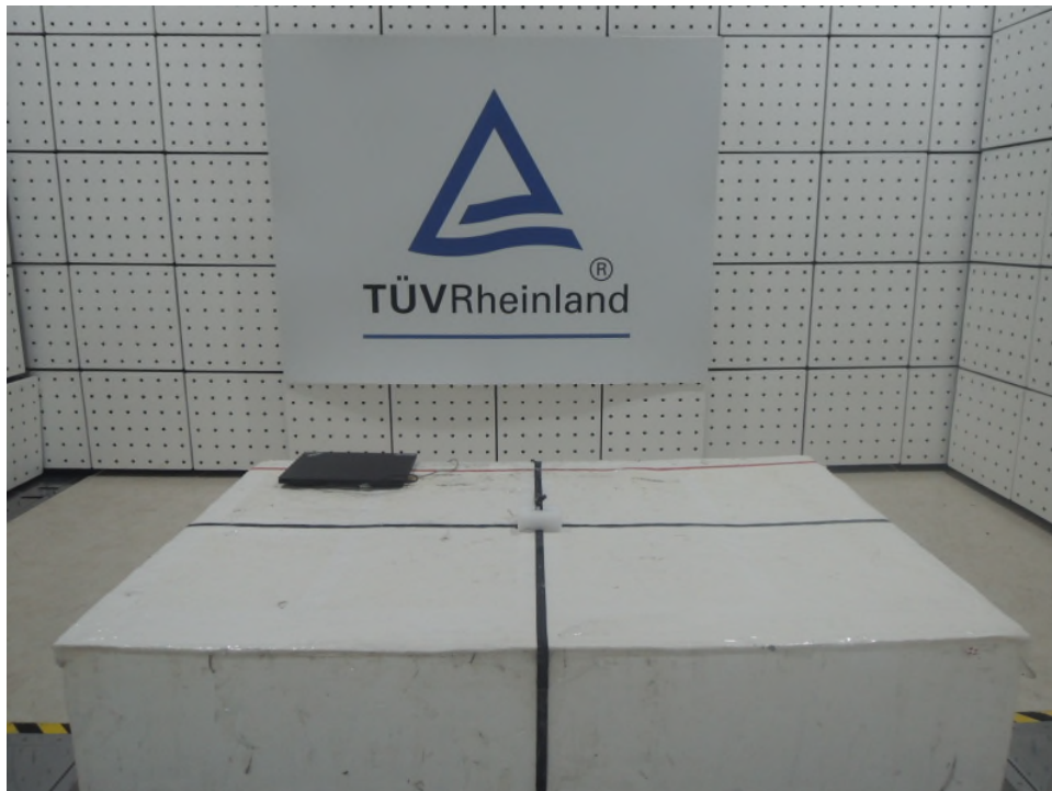
Photograph 1: Set-up for Spurious Emissions (Front View 1) – Left Ear
