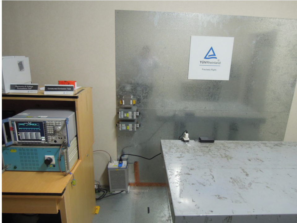
Photograph 17: Set-up for Mains Conducted testing (Front View)
