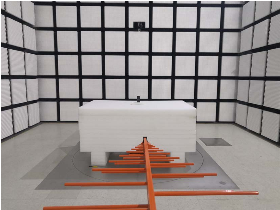
Radiated Emissions Below 1G View
