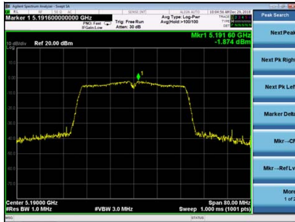
(802.11n40) PSD plot on channel 46
