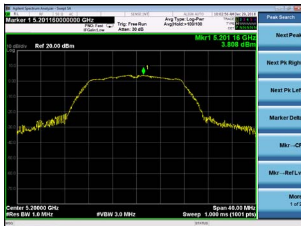
(802.11a) PSD plot on channel 48
