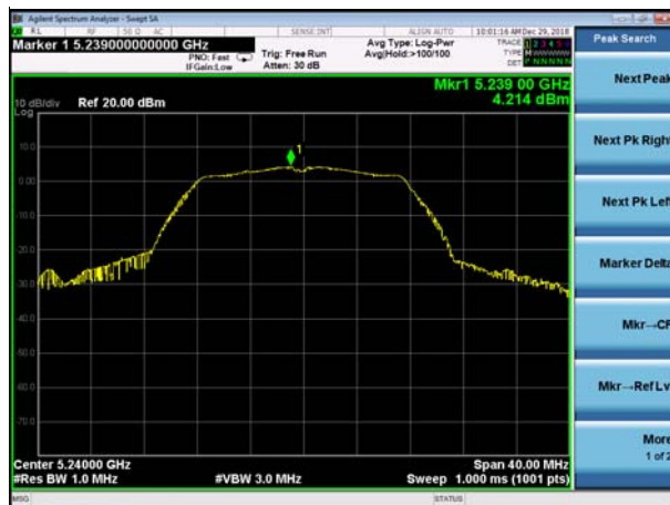
(802.11a) PSD plot on channel 48
