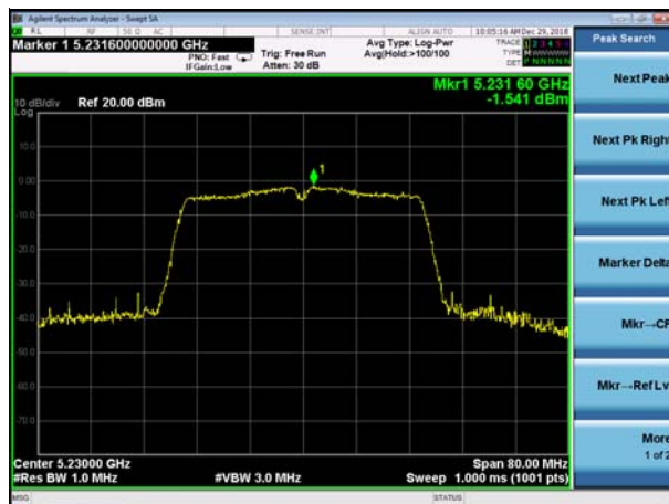
(802.11n40) PSD plot on channel 46
