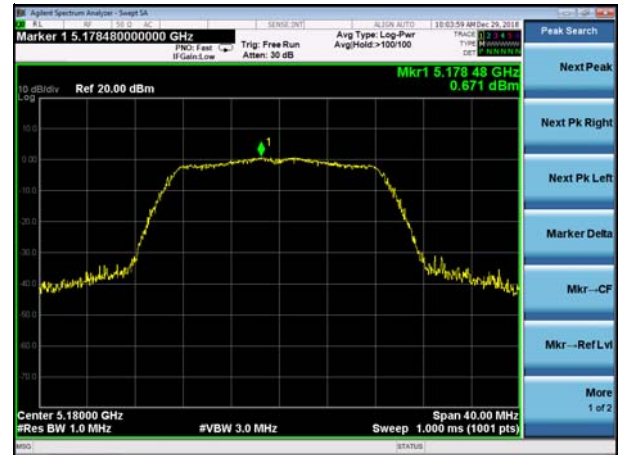
(802.11n20) PSD plot on channel 40
