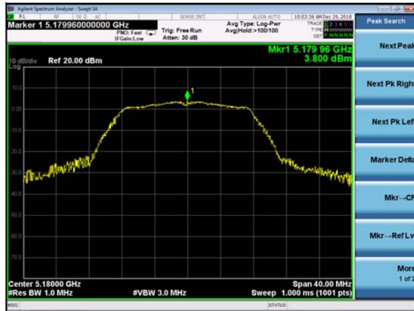
(802.11a) PSD plot on channel 40
