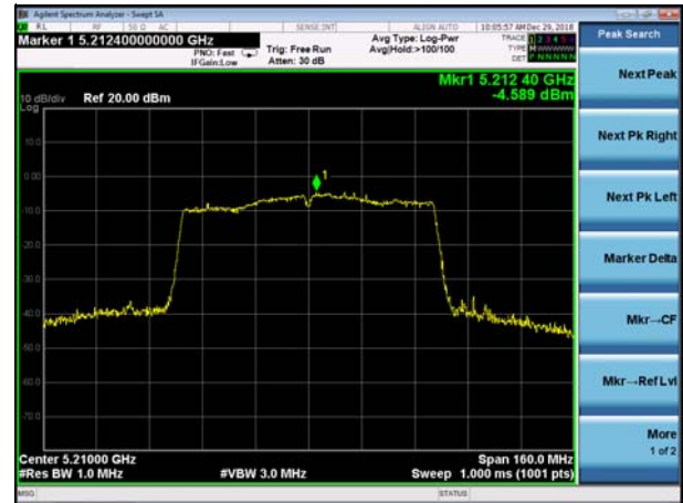
(802.11ac80) PSD plot on channel 42
