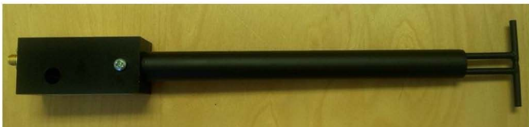
Figure 1 – MVG COMOSAR Validation Dipole
