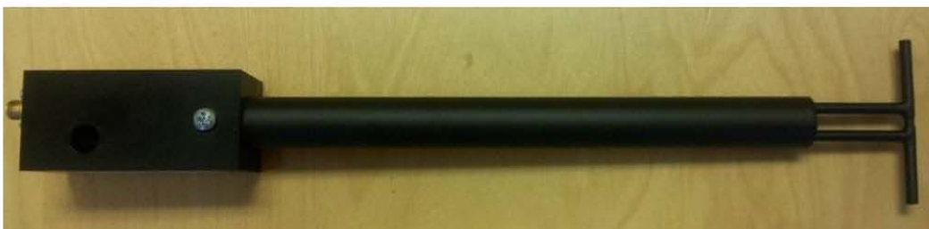
Figure 1 – MVG COMOSAR Validation Dipole
