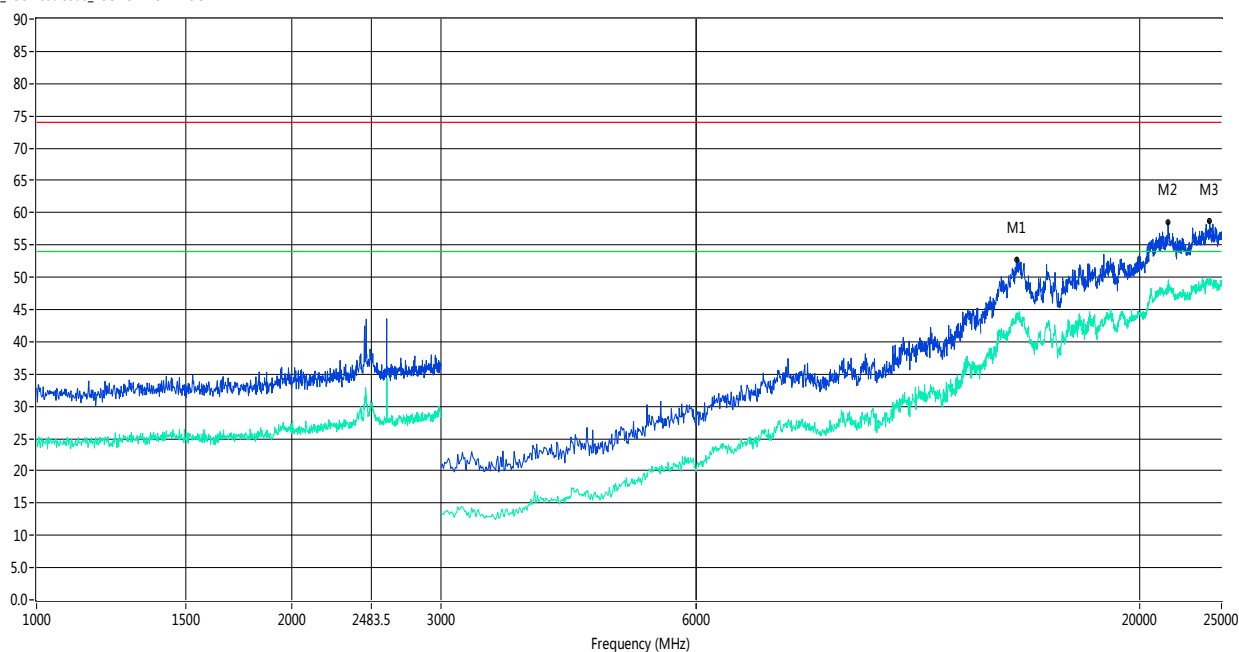
RE_FCC Test Case_FCC 15B 1GHz-25GHz
