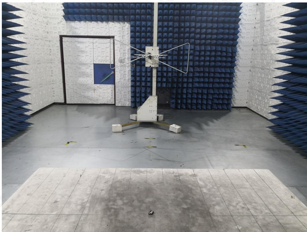
RADIATED EMISSION TEST SETUP ABOVE 1GHZ
