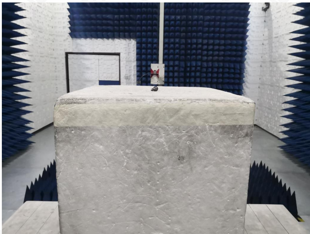
RADIATED EMISSION TEST SETUP ABOVE 1GHZ
