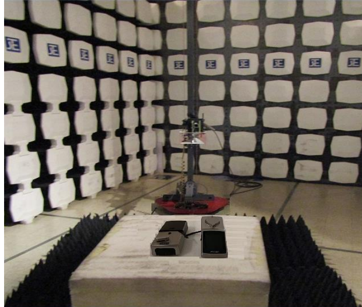
Measurement of Radiated Emission Test Set Up (Above 1000MHz)
