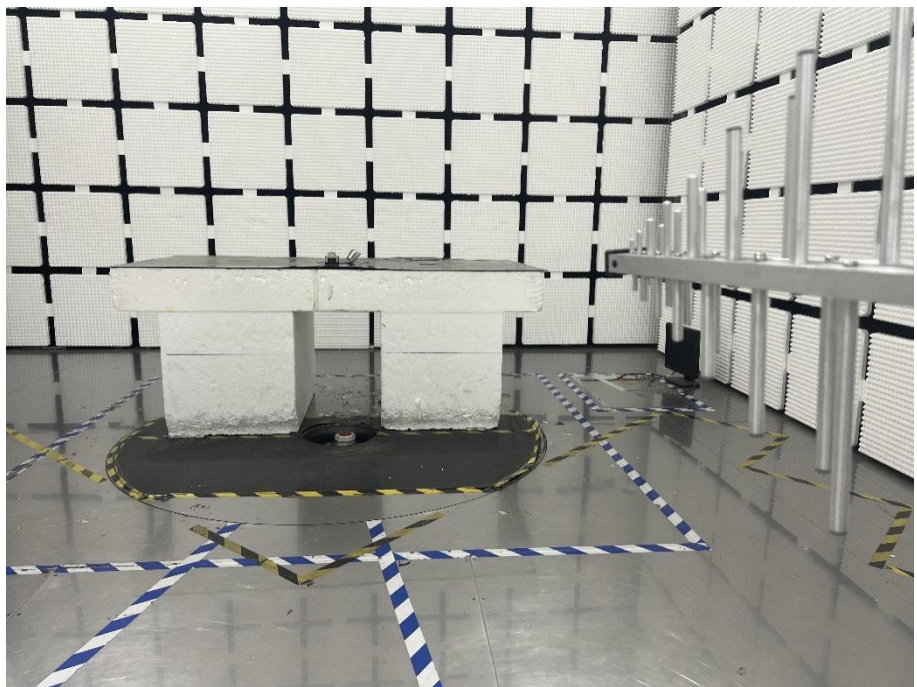
Radiation Emission Test Setup (30MHz to 1GHz)
