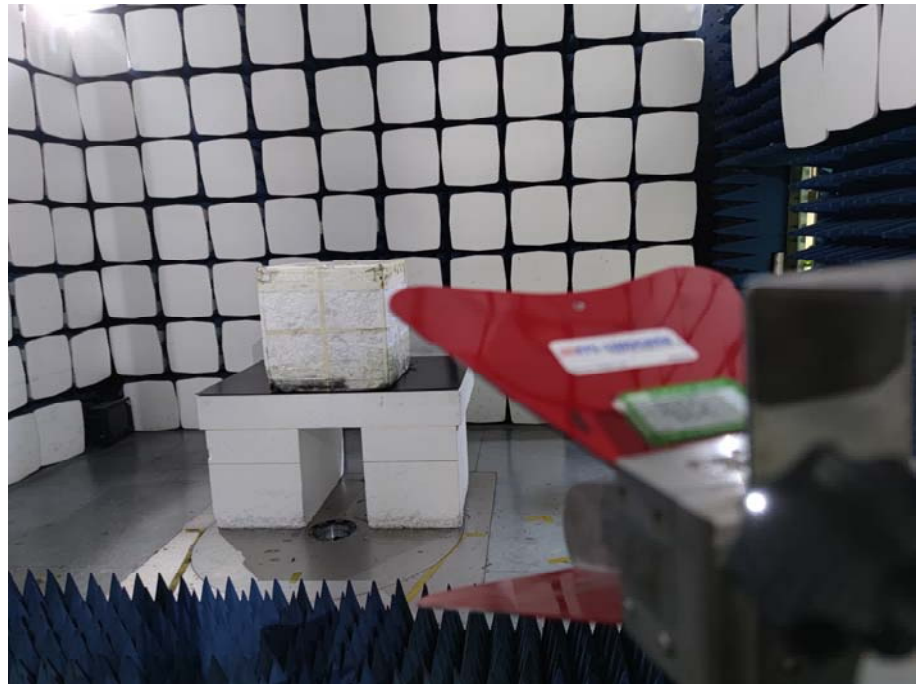
Radiation Emission Test Setup (1GHz to 18GHz)
