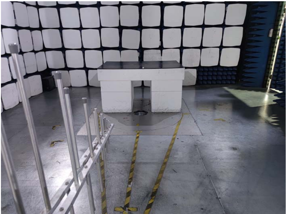
Radiation Emission Test Setup (30MHz to 1GHz)
