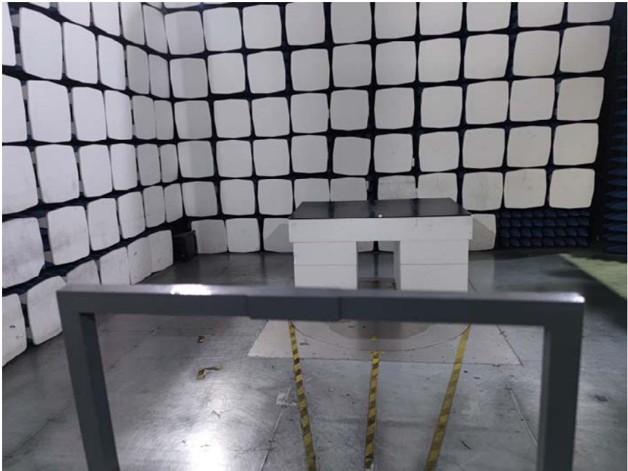
Radiation Emission Test Setup (Below 30MHz)
