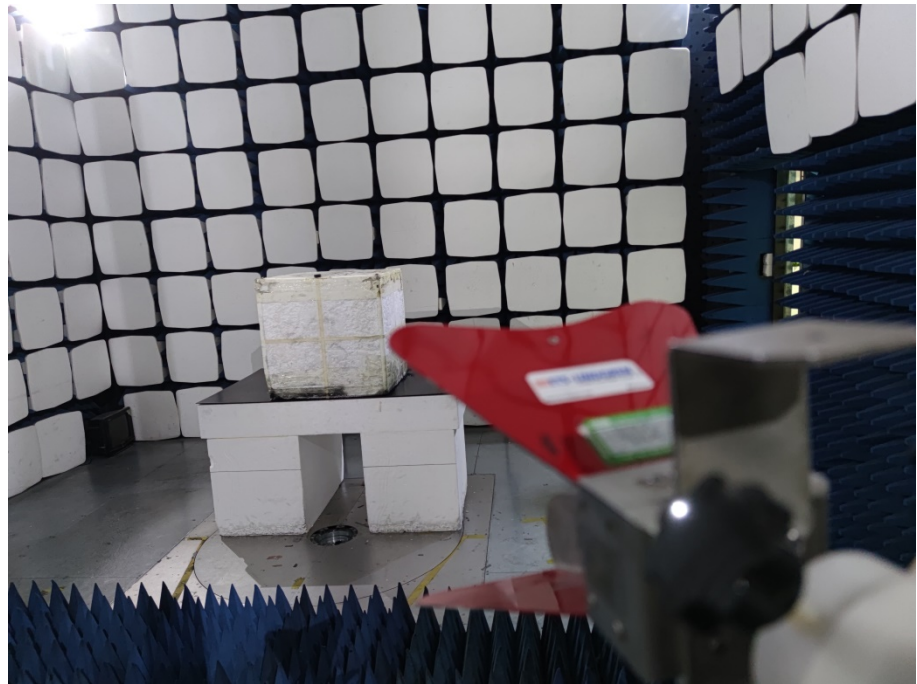
Radiation Emission Test Setup (1GHz to 18GHz)
