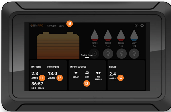
Figure 2: OdysseyControl Battery and Power Consumption
