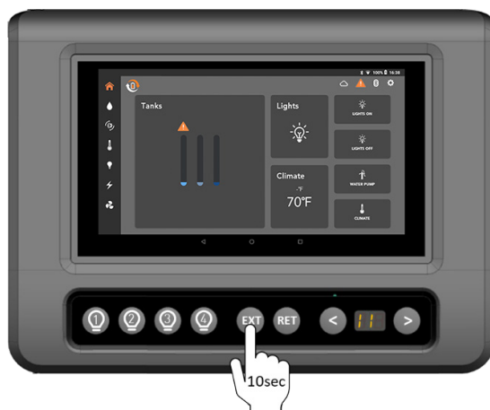
Figure 7: Navigate to 'PA' and press and hold EXT for 10 seconds to clear the Node memory
