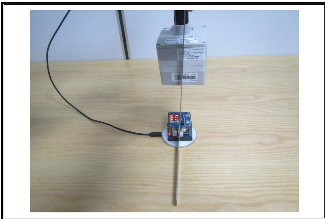
E-FIELD AND H- FIELD STRENGTH MEASUREMENT SETUP-5
