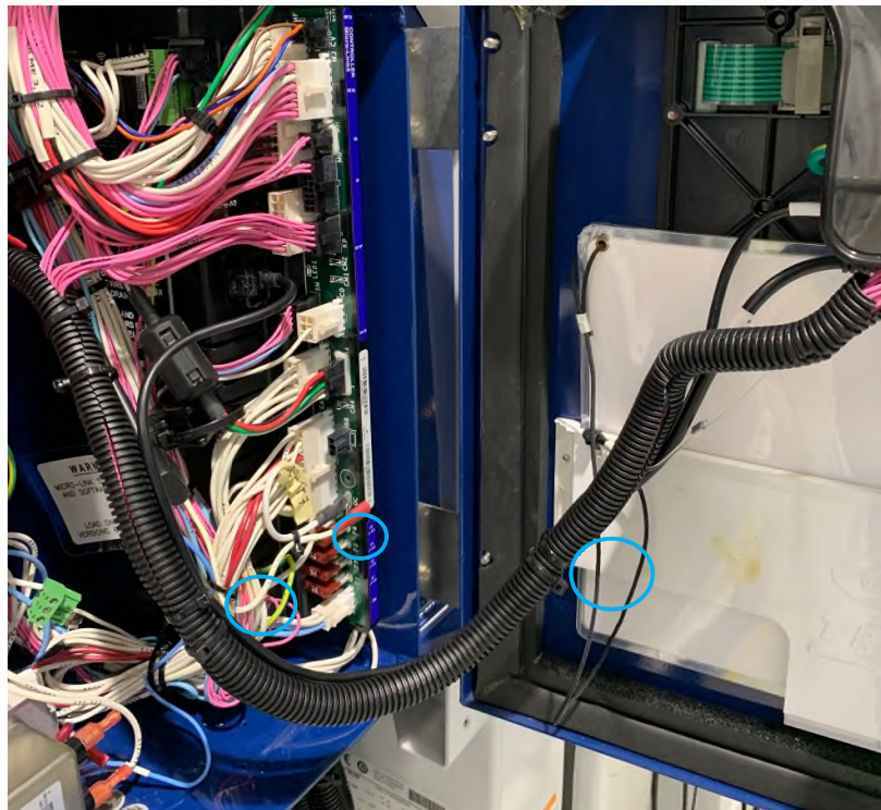
Figure 7a: Securing wire harness
