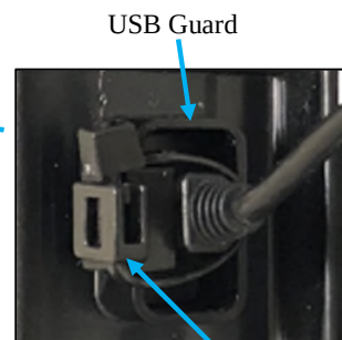
Figure 5c: STA-STRAP (item 4) Secure to USB guard
