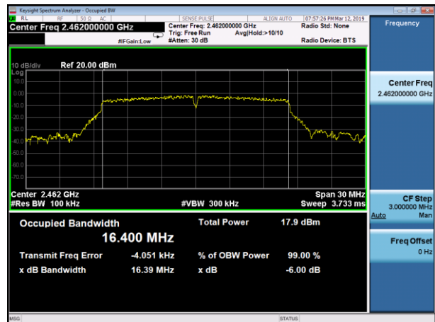
(802.11g) 6dB Bandwidth plot on channel 11
