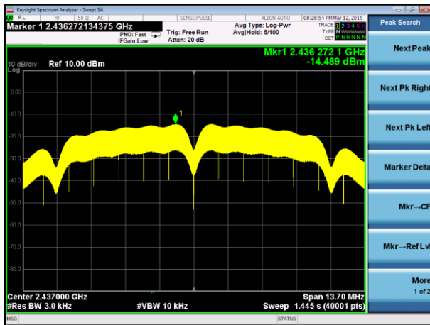
(802.11b) PSD plot on channel 11
