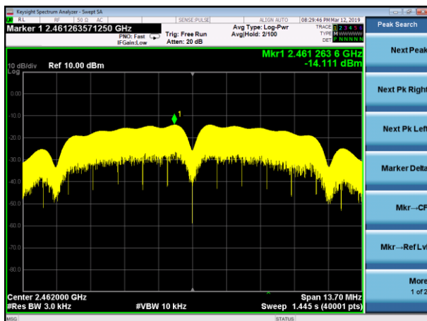
(802.11b) PSD plot on channel 11
