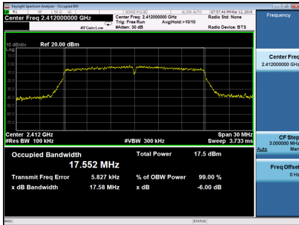
(802.11 N20) 6dB Bandwidth plot on channel 6
