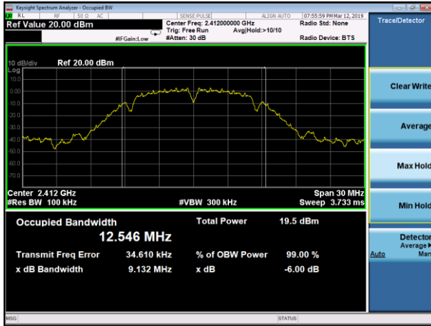
(802.11b) 6dB Bandwidth plot on channel 6
