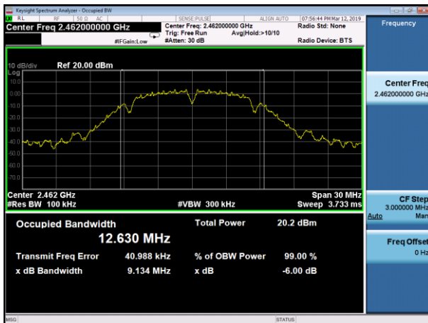
(802.11b) 6dB Bandwidth plot on channel 11
