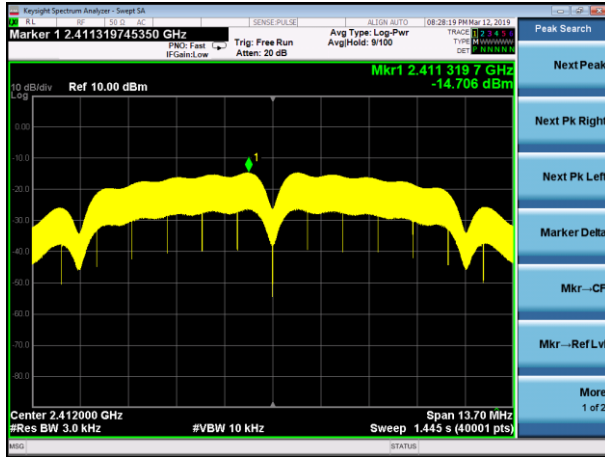
(802.11b) PSD plot on channel 6
