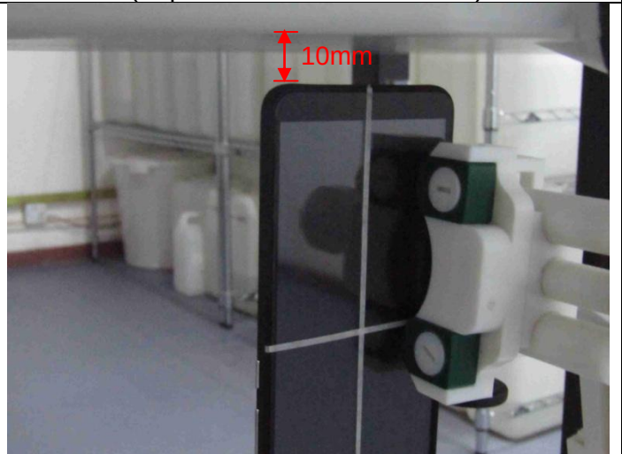
Bottom Side (Separation distance of 10mm)
