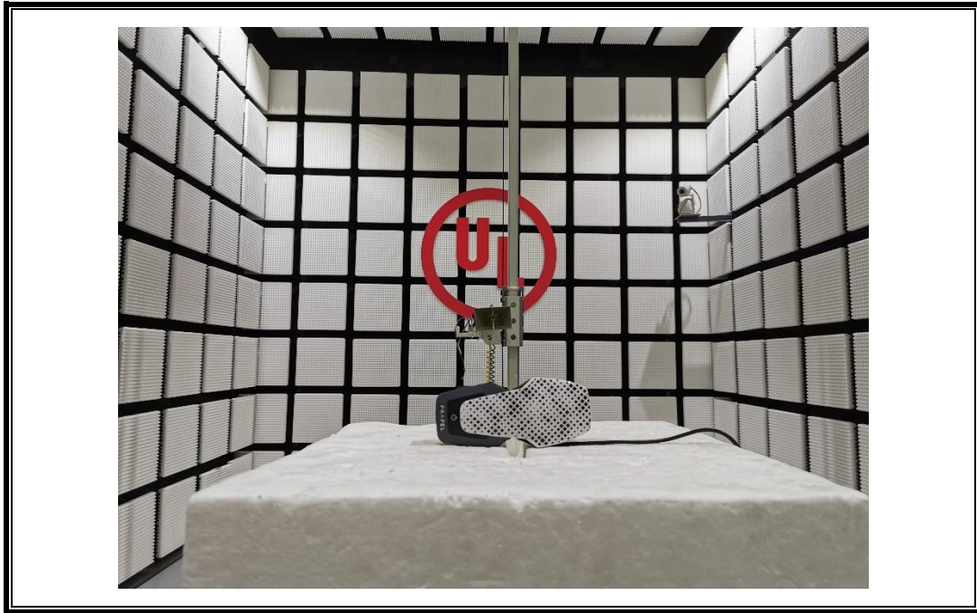
RADIATED RF MEASUREMENT SETUP for 2.4G WiFi function (Above 1G – Y axis)
