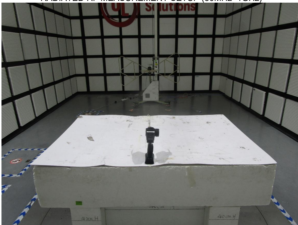
RADIATED RF MEASUREMENT SETUP (Below 30MHz)
