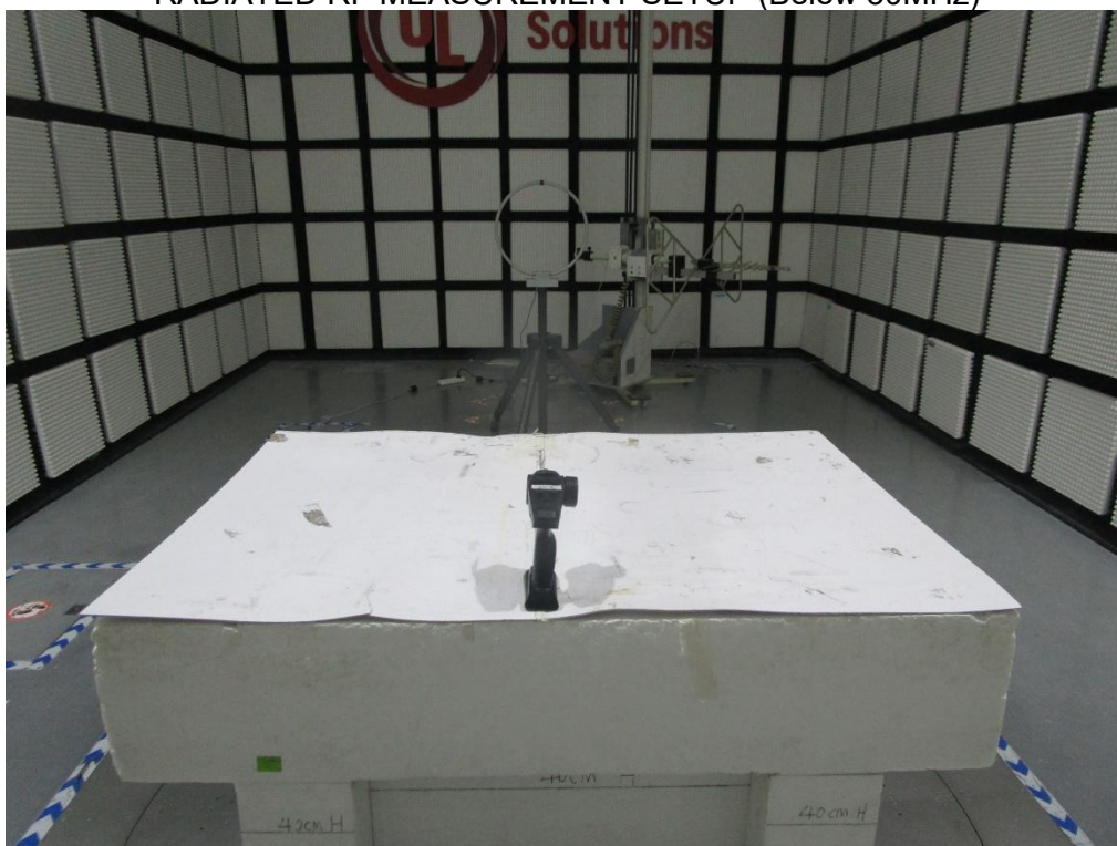
RADIATED RF MEASUREMENT SETUP (Below 30MHz)
