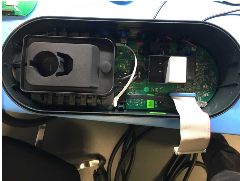
Photo 1: Casing and HPS board
