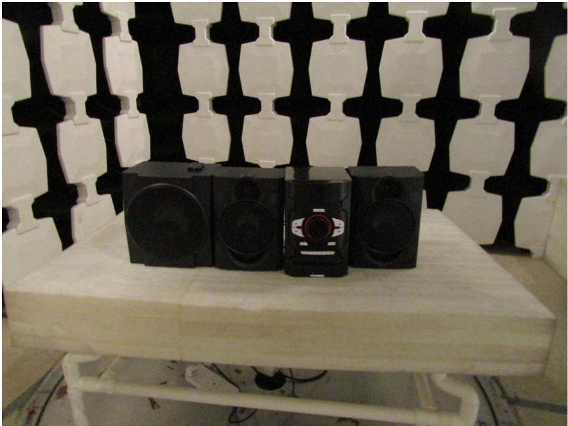
Measurement of Radiated Emission Test Set Up
