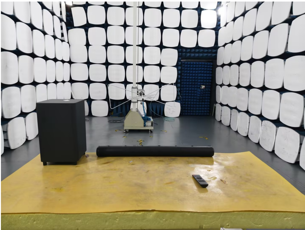
Radiated Spurious Emission, Above 1GHz
