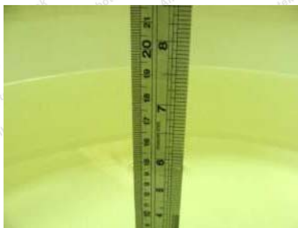
Photo of Liquid Height for Body SAR
