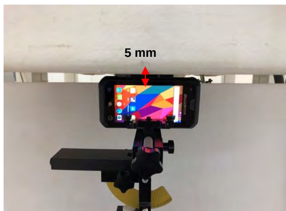
Fig.8 EUT Left side to flat phantom
