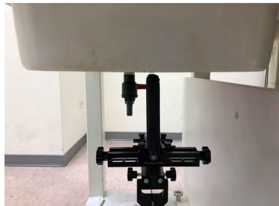
Fig.6 EUT Bottom side to flat phantom
