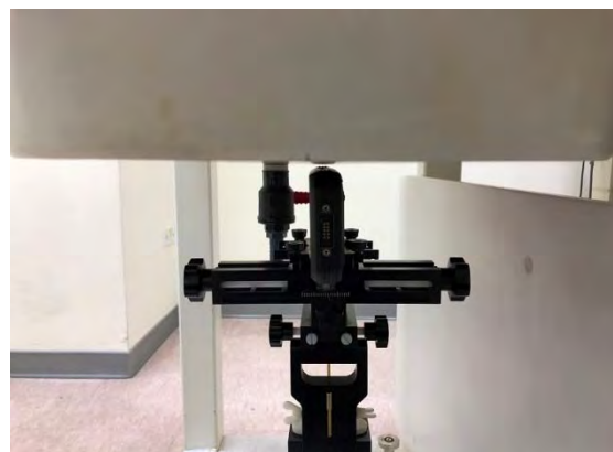
Fig.7 EUT Right side to flat phantom
