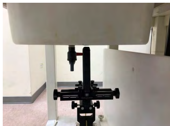
Fig.5 EUT Top side to flat phantom
