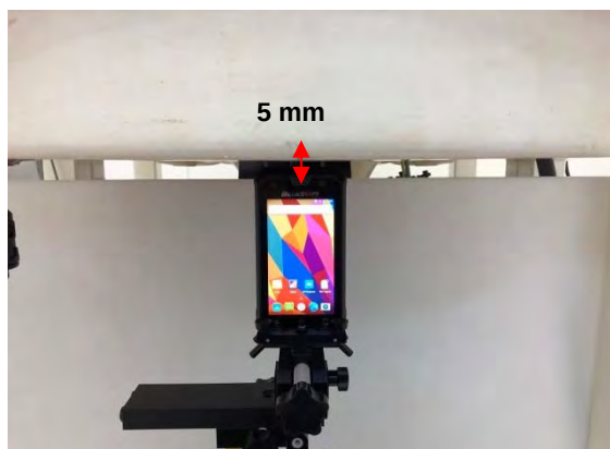
Fig.5 EUT Top side to flat phantom
