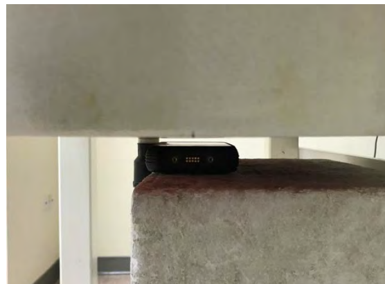
Fig.3 EUT Front side to flat phantom
