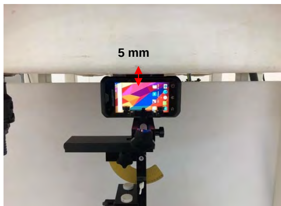
Fig.7 EUT Right side to flat phantom
