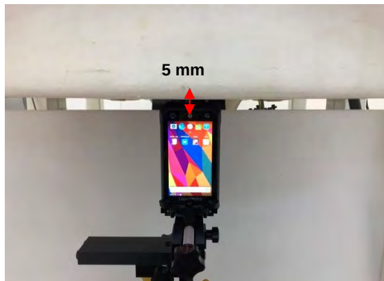
Fig.6 EUT Bottom side to flat phantom
