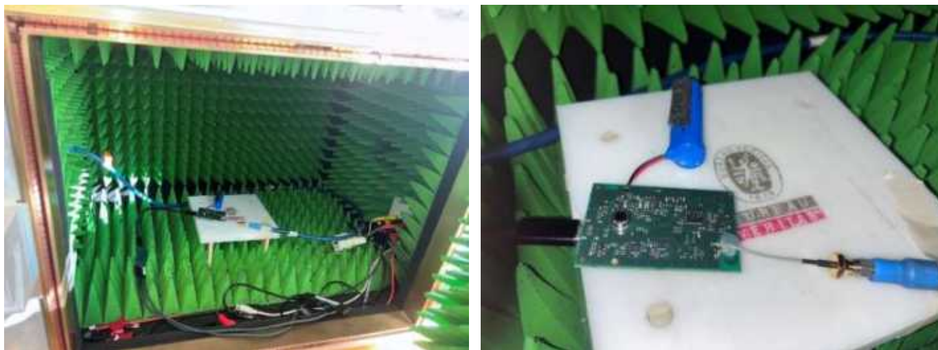
Photo of Maximum Conducted Output Power
